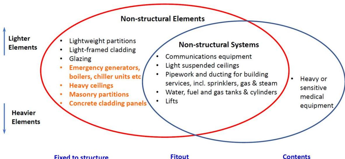
\* The elements in orange fall within the required scope of seismic assessments
